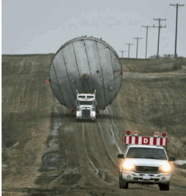
Talk about a road hog. SaskPower recently took part in the delivery of one of the largest stainless steel storage tanks ever to be shipped in Saskatchewan. The tank was 35 feet wide and weighed 60,000 lbs.
